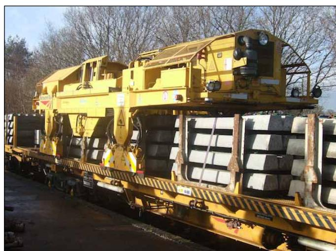
Figure 8. New concrete sleepers on the HOTR train alongside Bow Station on 16 January.
